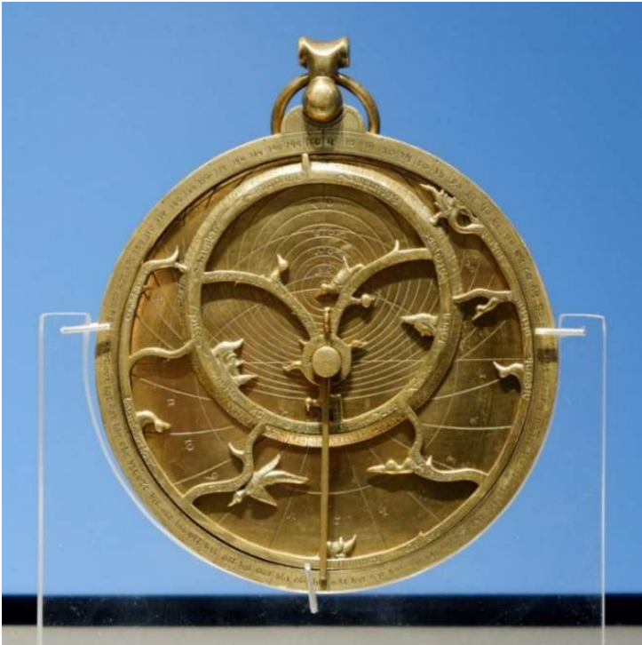
A rete, showing the cutaways, stars and star pointers, and the smaller, off-centre ecliptic ring. The lines of the latitude plate are visible underneath.
