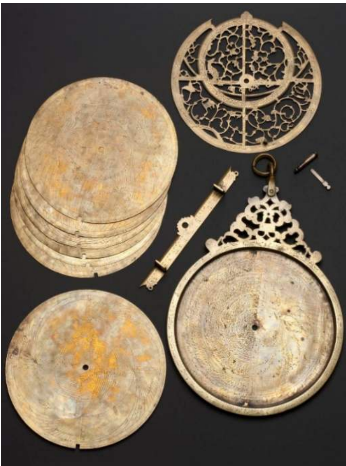
A rete, showing the cutaways, stars and star pointers, and the smaller, off-centre ecliptic ring. The lines of the latitude plate are visible underneath.
